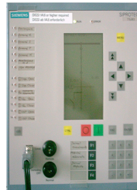
Fig. 6 SIPROTEC Siemens digital protection
